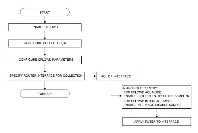
Figure 31: Cflowd Configuration and Implementation Flow
